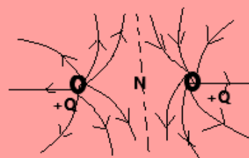
Figure-5(2): Electric Field Lines due to two like charges of equal magnitude
